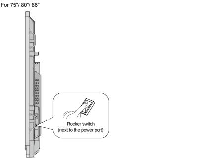
Step 3: Press power switch on the control panel or **Power** on the remote controller to turn on the interactive touch screen. The OPS is boot. The power indicator turns green.
