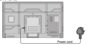
Step 2: Connect the screen to the power supply. Switch on the rocker switch (on the right bottom of the rear of the screen, next to the power port) to enter the standby status. The power indicator turns red.
