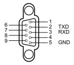
Connect RS-232 port to the PC or controlling device. Enable RS-232 serial port connection and complete the following configuration.
