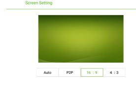
• Under AV signal source, the P2P mode cannot use.
