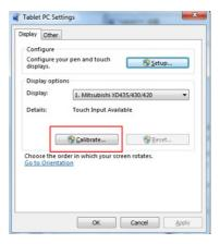
Step 4: Use the pen to click and hold the center of the flickering cross. Do not release it until the flickering cross moves to the next point. Repeat and complete the positioning process according to instructions on the interface.
