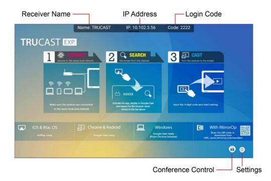
You will see the following information on the standby screen: (a) receiver name (name of the receiver device with the TRUCAST app installed); (b) IP address of the receiver device; (c) login code/passcode (if a code is set on the receiver device); (d) a quick guide on how to use TRUCAST; (e) available casting options.
