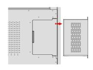
Step 2: Push the internal PC into the port at the rear of the screen from right to left.
