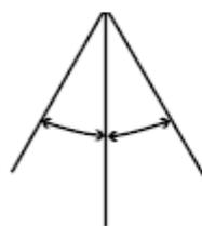
The effective receiving area is about 3 meters with 30° angle from vertical point to the right.
