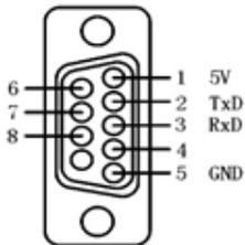
Connect RS-232 port to the PC or controlling device. Enable RS-232 serial port connection and complete the following configuration.
