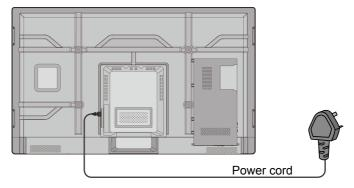
Step 2: Connect the display to the power supply. Switch on the rocker switch (on the right bottom of the rear of the display, next to the power port) to enter the standby status. The power indicator turns red.
