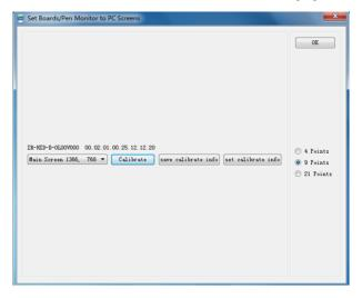
Step 4: Use the pen to click and hold the center of the flickering cross. Do not release it until the flickering cross moves to the next point. Repeat and complete the positioning process according to the instructions on the interface. The software interface returns to the desktop automatically after the positioning is completed successfully.
