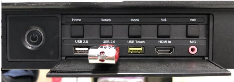
Step 3: Press down “Menu” button, DO NOT release, and then switch on screen, the main firmware upgrade will start automatically, then release menu button.
