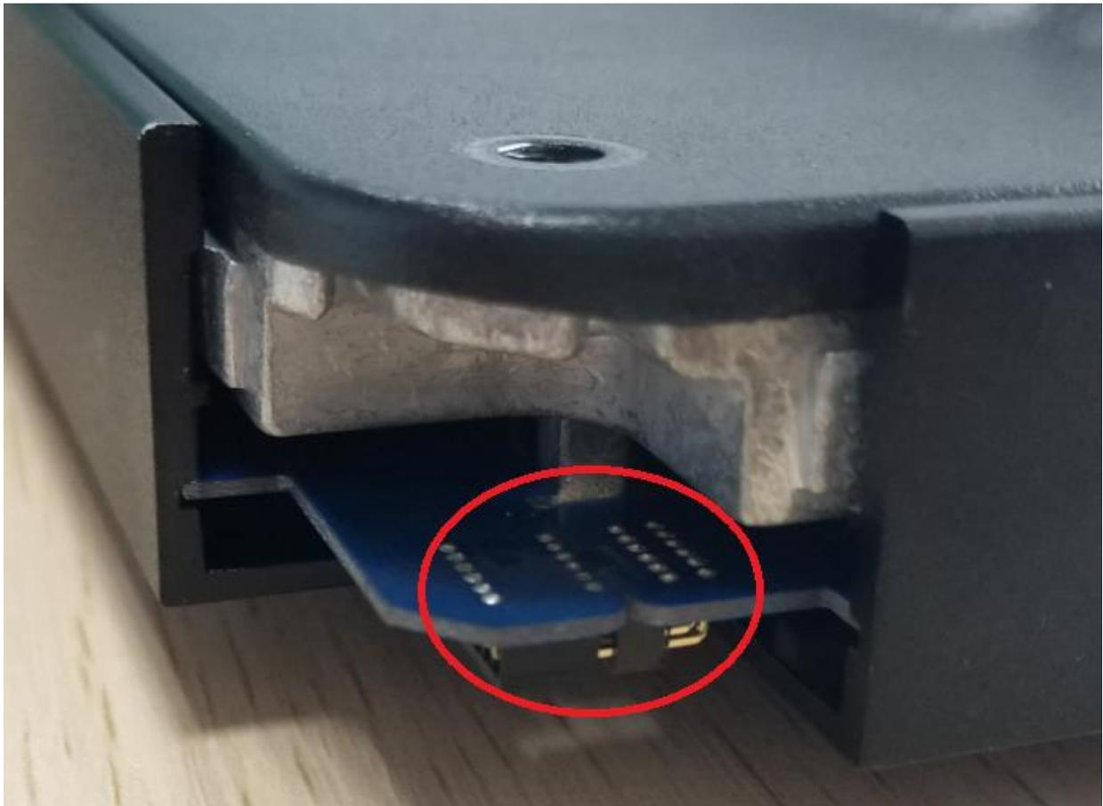
Step 2. Use a thin screwdriver or ball-pen to push and disconnect the PCBAs in the corner then take out the disconnected PCBA according to below red mark direction.
