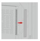
Step 2: Push the internal PC horizontally into the interface card slot.
