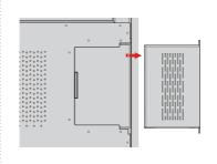
Step 2: Push the internal into the internal PC port at the rear of the screen from right to left.
