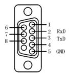
Connect RS-232 port to the PC or controlling device. Enable RS-233 serial port connection and complete the following configuration.
