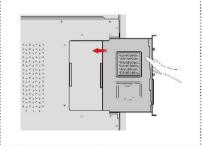
Step 3: Secure the internal PC to the display by using the M3 screws.
