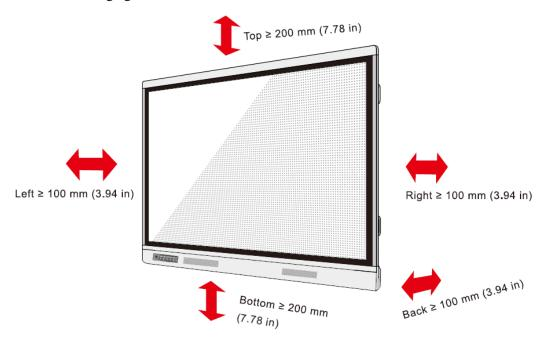
Ensure adequate ventilation and/or an air conditioned environment. We recommend keeping certain distances from the side of the product to the wall or panels. Ventilation requirements are shown in following figure:
