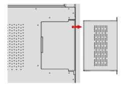
Step 2 Push the internal PC into the port at the rear of the screen from right to left.
