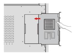
Step 3 Secure the internal PC to the display by using the M3 screws.
