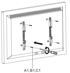
Notes: Plastic spacers must be used (except for C2) when assemble adaptor ontoyour display to avoid display threadedholes damaged when threadholes are shallow.
