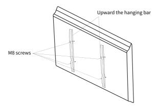
3. Equipment Installation: Hang the equipment with the hanging bar into the wallboard, fine adjust the position and angle to ensure the stability of the equipment.
