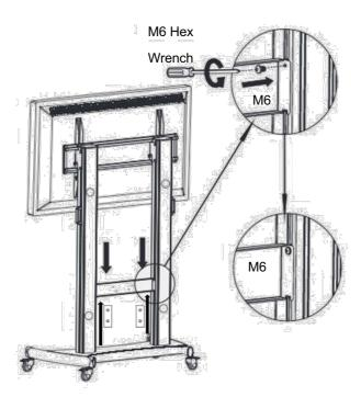
After sliding the 2-hole fixed iron piece to a proper height, lock the horizontal pillar. At the same time make sure the horizontal pillar is horizontal.
