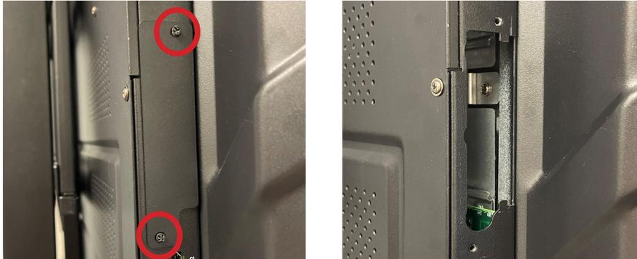
2. Insert the Wi-Fi Module into the port on the rear of the panel until firmly seated, using the 2 screws to secure it.
