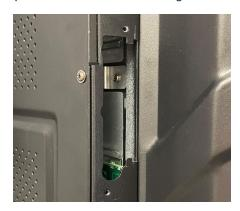
2. Insert the Wi-Fi Module into the port on the rear of the panel until firmly seated, using the 2 screws to secure it.
