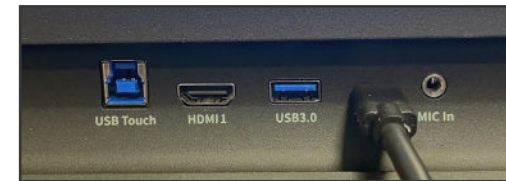
Front Ports with USB Type-C cable connected.
