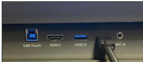
Front Ports with USB Type-C cable connected.
