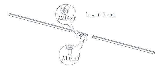
5. Assembly the right side and left side of "A" shape stand with the lower beams
