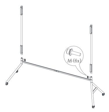
7. Connect the upper beam to the right and left castor bases, as shown below:
