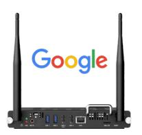
Part Number RK3588 CPU Quad-core Cortex-A55 GPU Mali-G52-2EE Storage 64GB eMMC RAM 8GB Built-in WiFi WiFi 6 2.4GHz + 5GHz Bluetooth 5.2 Bluetooth os Android 12
