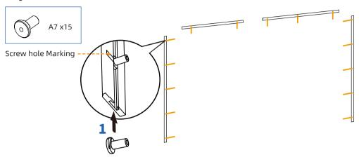
Next, insert the corner covers into the left side of the upper left frame and the right side of the upper right frame, as indicated by the figure.
