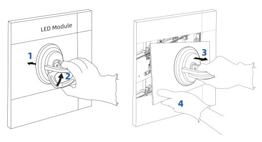
Notes: Make sure that the module does not touch the adjacent modules when pulling out, so as to avoid collision and damage to the other modules or LEDs.
