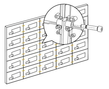
After completing the cabinet installation, use two A9 Hexagon socket bolts to lock the ends of the upper wall bracket.
