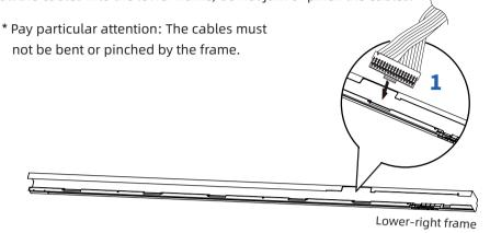
Secure the lower frame using A6 Hexagon socket bolts from top to bottom. Secure the lower-right frame first, then the lower-left frame, ensuring that the installation is flush.
