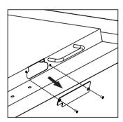
Step 2: Insert the Wi-Fi Module into the port on the rear of the LED display until firmly seated, using the 2 screws to secure it.
