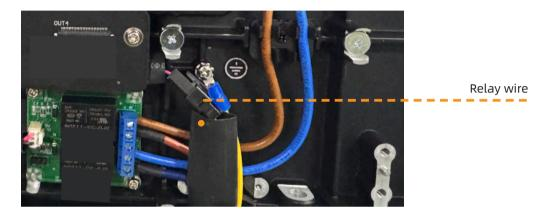
Step 3. Connect the power lines, numbered Line 1-5, to the E1-A1 cabinet in sequence:
