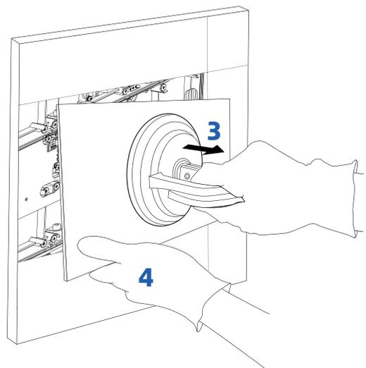
Notes: Make sure that the module does not touch the adjacent modules when pulling out, so as to avoid collision and damage to the other modules or LEDs.
