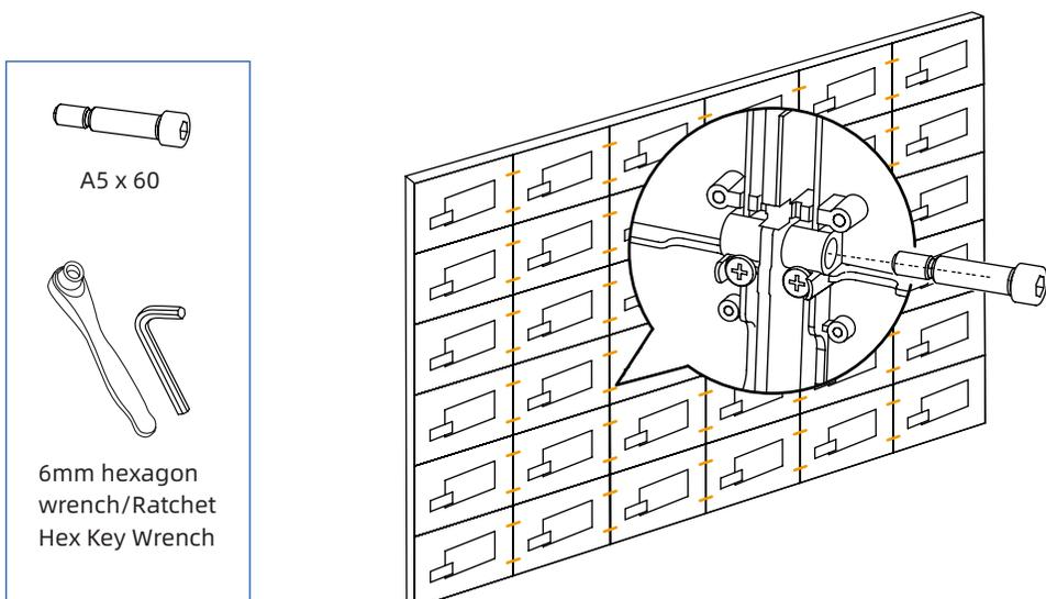
After completing the cabinet installation, use two A9 Hexagon socket bolts to lock the ends of the upper wall bracket.
