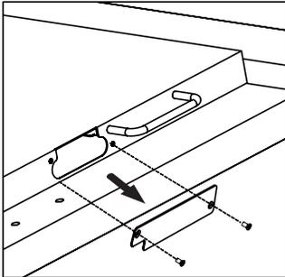
Step 2: Insert the Wi-Fi Module into the port on the rear of the LED display until firmly seated, using the 2 screws to secure it.
