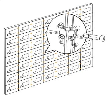
After completing the cabinet installation, use two A9 Hexagon socket bolts to lock the ends of the upper wall bracket.
