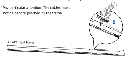
Secure the lower frame using A6 Hexagon socket bolts from top to bottom. Secure the lower-right frame first, then the lower-middle frame second, at last the lower-left frame, ensuring that the installation is flush.
