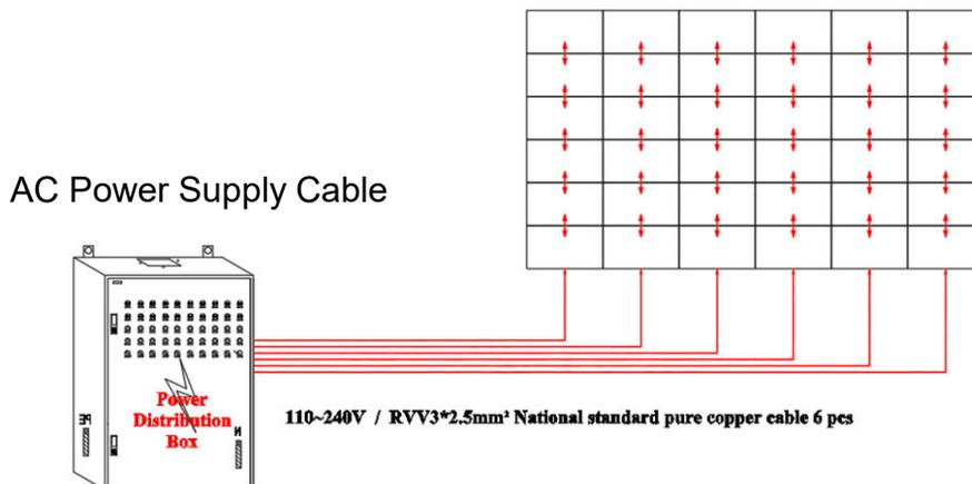
Fig 2-22 Power Cable Connection Diagram of P0.9
