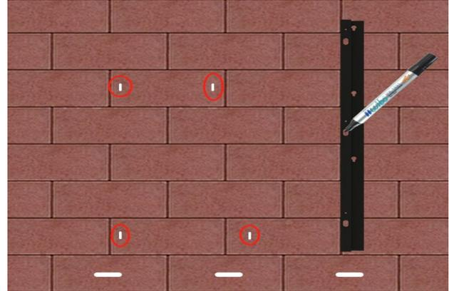
2. Position the wall mount according to the horizontal mark, ensuring the screws are properly aligned and marked.
