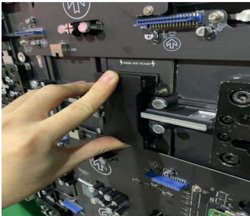
7. Install the power connector between the cabinets
