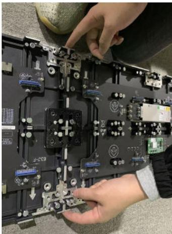
3. Ensure that the top and bottom are level, with a tolerance of no more than  $\pm 0.1\text{mm}$ .
