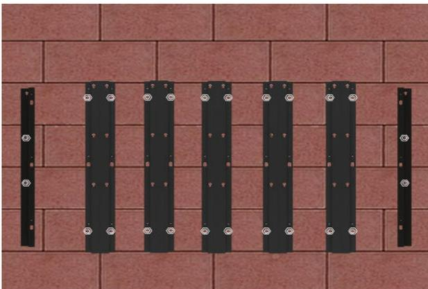
3. Use expansion screws to secure the marked points.
