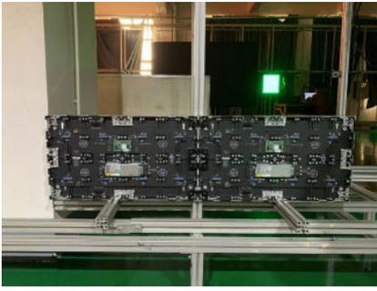
5. Place the cabinets on the ground, ensuring that their centers are level with the square tube.
