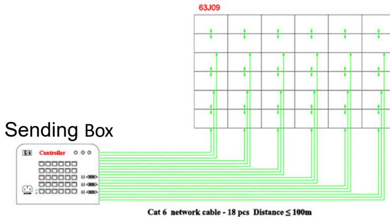
Fig 2-21 Signal Cable Connection Diagram of P0.9
