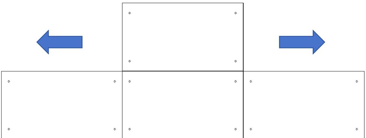
7. For multiple cabinets, secure them from the center first, then install the left and right sides.
