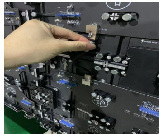
8. Install short network cables between cabinets
