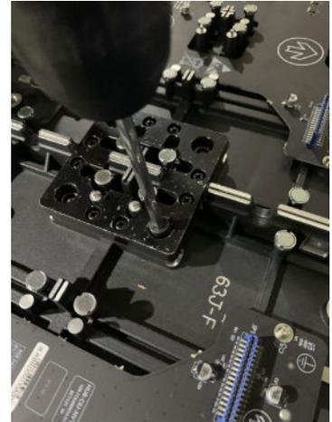
2. Use a hexagon socket wrench to tighten the screws.
