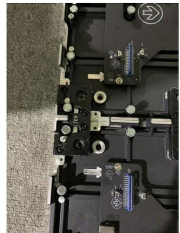
4. Proceed to connect the lower piece and secure it in place.
