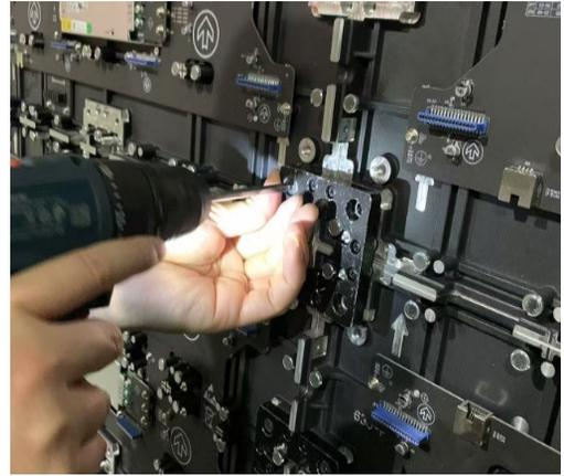
6. Use M5 screws to secure the connection, ensuring that the top and bottom are level. The tolerance must be within  $\pm 0.1\text{mm}$ .
