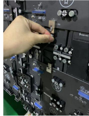
11. Install the short network cables between the cabinets.
