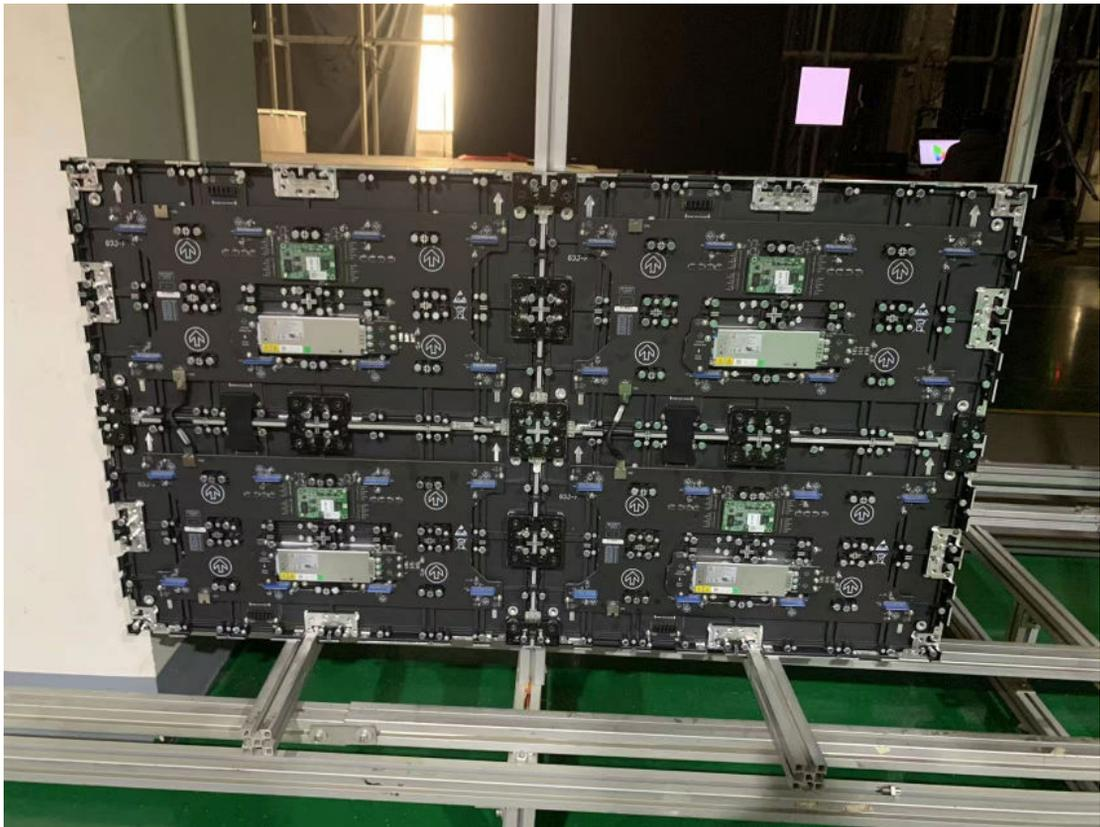
11. After installing the connector, verify the flatness of the connection and ensure the signal cable is properly connected. Once confirmed, connect the long signal cable and the long power cable according to the installation diagram.
