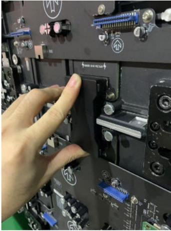
10. Install the power connector between the cabinets.
