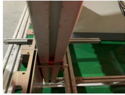
6. Use the long connecting pieces and hexagon screws to secure the cabinet to the square tube.
