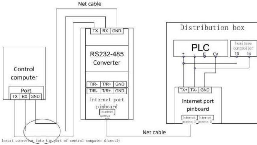
Fig 2-26 Distribution Box PLC Connection Diagram
