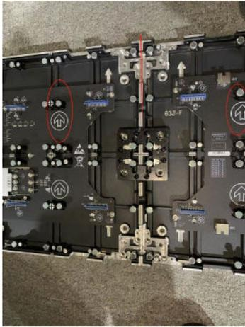
1. Pay attention to the direction of the arrow on the cabinet. Ensure that the cabinets are level and install the connecting piece accordingly
